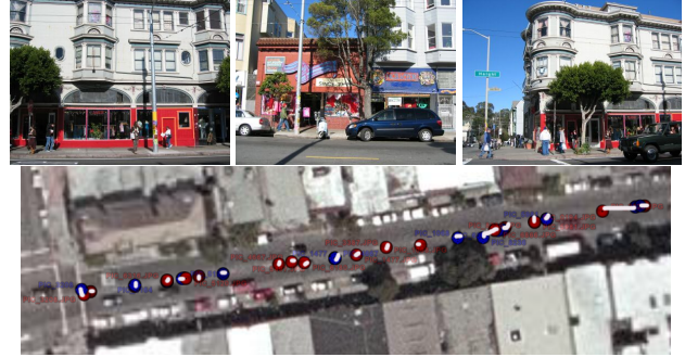
Figure 8. Top: Images with unknown GPS location for Test4. Bottom: GPS locations (blue) obtained using our method is compared with ground truth GPS (red). The white lines show the distance between the estimated and actual GPS locations.
