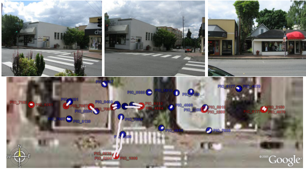
Figure 9. Top: Images with unknown GPS location for Final5. Bottom: GPS locations (blue) obtained using our method is compared with ground truth GPS (red). The white lines show the distance between the estimated and actual GPS locations.
