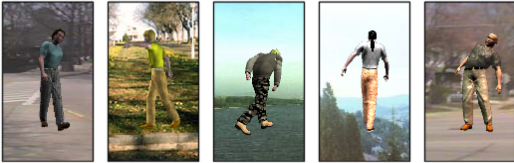
Figure 4.5: Sample images from the superimpose program. Each image is 96x160 pixels. Each image has a 16 pixel margin around the centered 64x128 sample window and an approximate border size of 16 pixel between the figure and centered 64x128 sample window.
