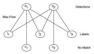
Figure 9. Maximum weight matching in a bipartite graph. We make an injective (one-to-one) mapping from the set of detected image regions  $d_i$  to the set of image regions  $l_i$  annotated as face regions. The property of the resulting mapping is that it maximizes the cumulative similarity score for all the detected image regions.
