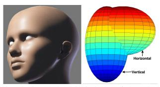
Figure 5. *Shape of a human head*. The shape of a human head (**left**) can be approximated as the union of two ellipsoids (**right**). We refer to these ellipses as vertical and horizontal ellipsoids.
