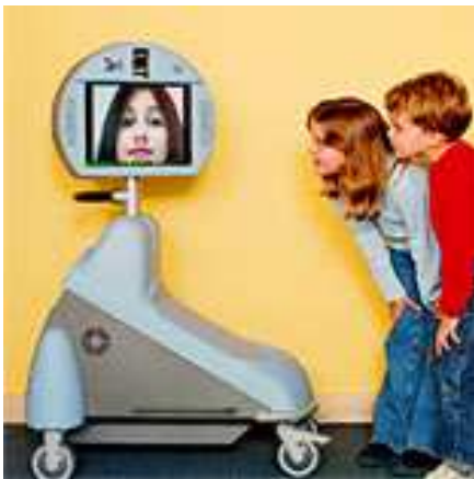
Figure 3: Pebbles is a mobile teleconferencing application that attends school for disabled children—allowing them to maintain relationships with their peers. Pebbles includes a rudimentary manipulator for interacting with the teacher in the classroom setting.
