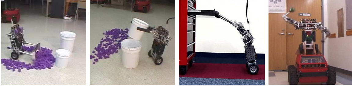
Figure 8: The uBot-4 performing plowing, stacking, pushing, and throwing tasks.
