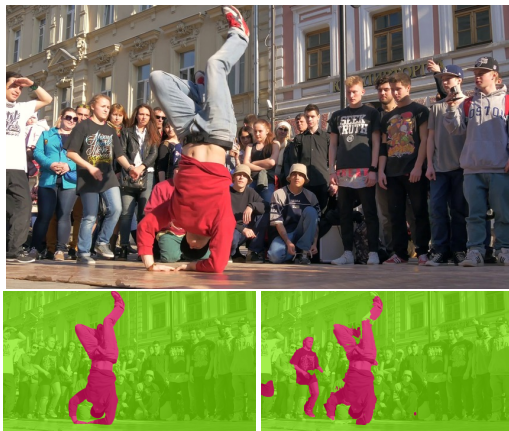
Figure 3: Segmentation on DAVIS. Segmentation of the breakdance video sequence (frame 2). Bottom left: ground truth, bottom right: motion segmentation. An evaluation on DAVIS doesn’t mirror necessarily the quality of the motion segmentation method. A motion segmentation method is accurate if all moving objects are segmented, irrespectively whether they are the primary object of interest or not.
