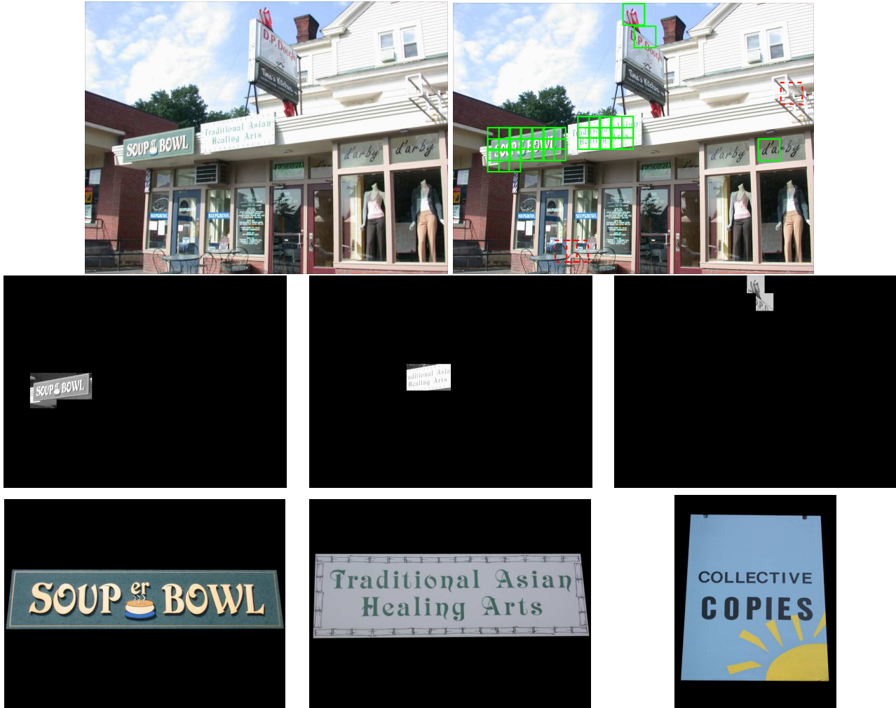
Figure 8. A sample result after integrating the detector and recognizer. The first row contains the initial image and the result of the detector. The second row shows sample results of three connected components and their respective segmentation. The third row shows the result of matching each connected component with the sign classes in the 65 sign data set. The third sign was classified incorrectly because the image region does not belong to any of the signs in the database. However, our trained meta-classifier successfully classified the image region as a negative instance, meaning that it does not belong to any of the classes in the database.
