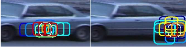
Figure 7: Patch Correlations . On each image, the patches most correlated with the white-circled patch are shown. Notice that in the left image, where the patch sits in an area with a highly visible horizontal structure, the most correlated patches all lie along the horizontal features. Contrast this with the right image, showing correlation of patches with a patch sitting on a wheel, where the most correlated patches are those that strictly overlap the white-circled patch.
