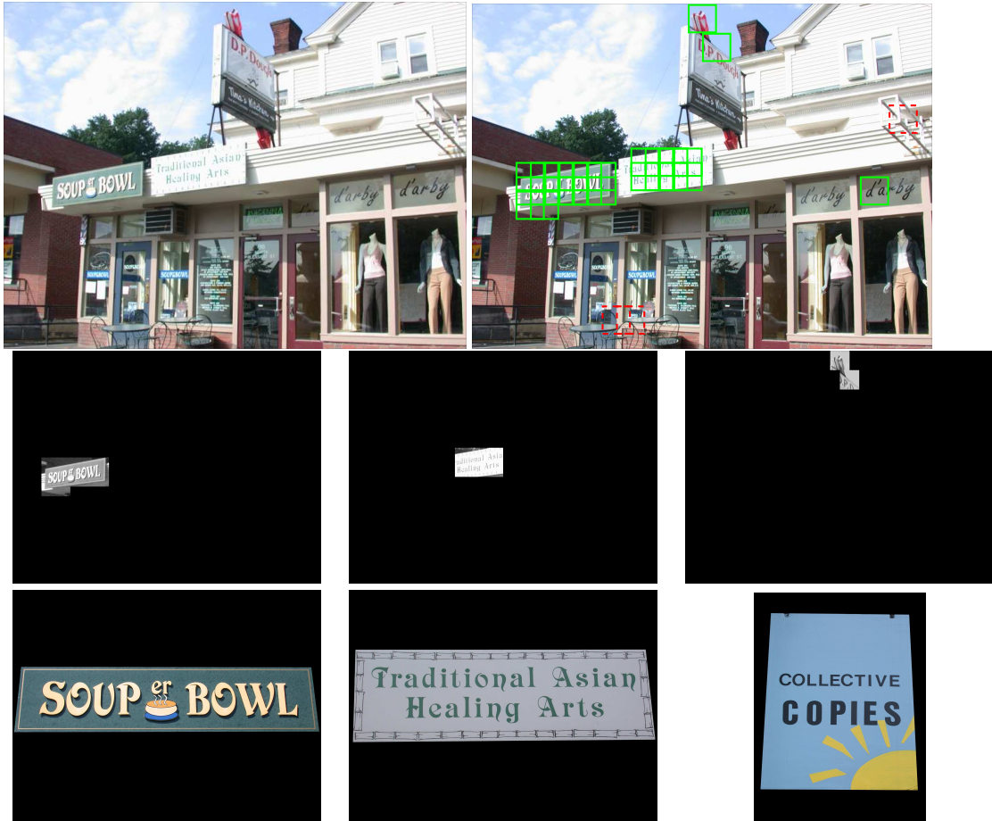
Figure 9: A sample result after integrating the detector and recognizer. The first row contains the initial image and the result of the detector. The second row shows sample results of three connected components and their respective segmentation. The third row shows the result of matching each connected component with the sign classes in the 65 sign data set. The third sign was classified incorrectly because the image region does not belong to any of the signs in the database. However, our trained meta-classifier successfully classified the image region as a negative instance, meaning that it does not belong to any of the classes in the database.
