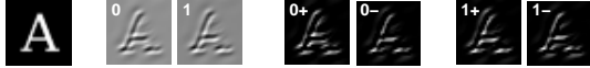
Figure 3. An image is transformed by the steerable pyramid and rectified. For one orientation, the responses of even (0) and odd (1) filters for one orientation along with their positive (+) and negative (-) rectified components are shown.
